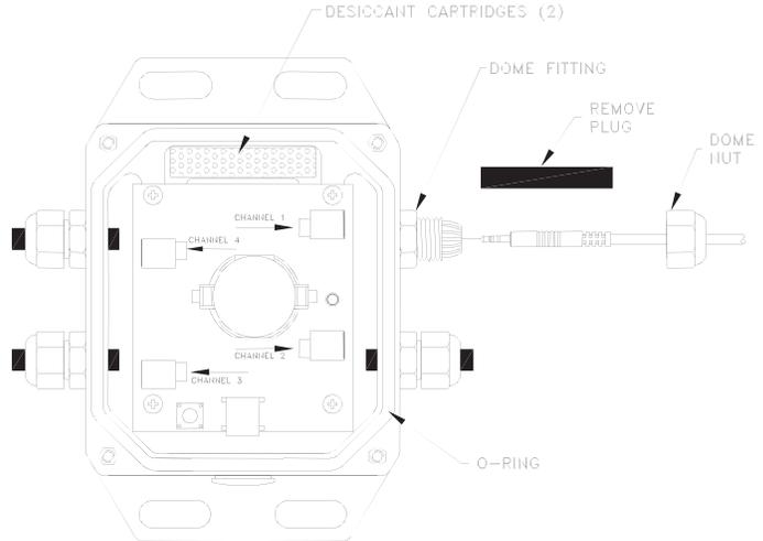
6. Thread the dome nut back onto fitting and hand-tighten it. Tighten an additional half-turn with a 15 mm wrench.
