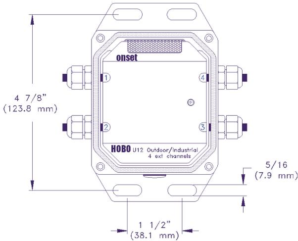
U-bolt clamps (part # U-BOLT-KIT) are preferred for mounting to a 1" pipe (1.3" outside diameter), as shown.
