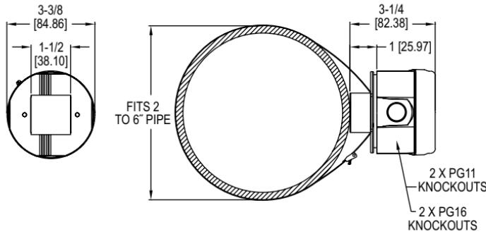
The Series TE-SNW Weather Resistant Surface Temperature Sensor non-intrusively measures the process temperature in hot and cold water loops in buildings. In order to work with most common building controllers, the output of the sensor can be chosen from 6 different RTD and Thermistor curves.
