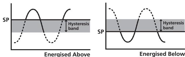
*CNTRL - SP VALUE controls setpoint deactivation point. HYSTERESIS VALUE controls setpoint reactivation point.*
