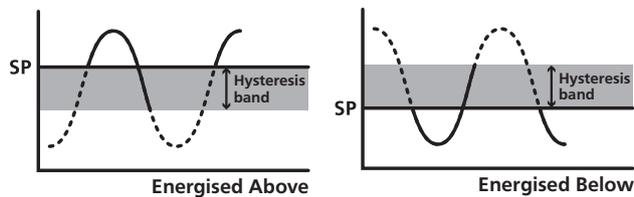
***CTRL - SETPOINT VALUE** controls setpoint deactivation point. **HYSTERESIS VALUE** controls setpoint reactivation point.*
