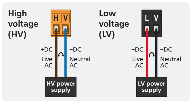
Once you have completed the wiring process it is safe to switch on your power supply. Ensure that your display is functioning before you proceed.
