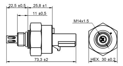
All dimensions are millimeters (mm). Mating connector type is FCI female receptacle ref. 54200409 (black-sealed). Sensor body is stainless steel.
