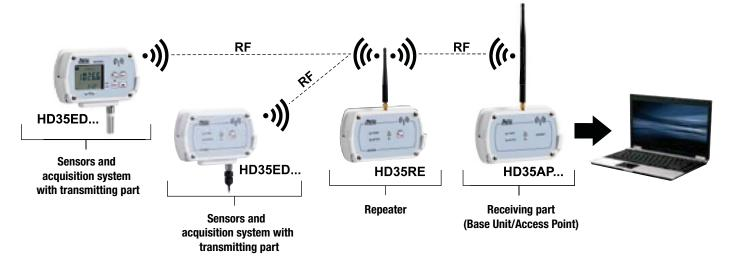
Wireless data recording system with repeater
